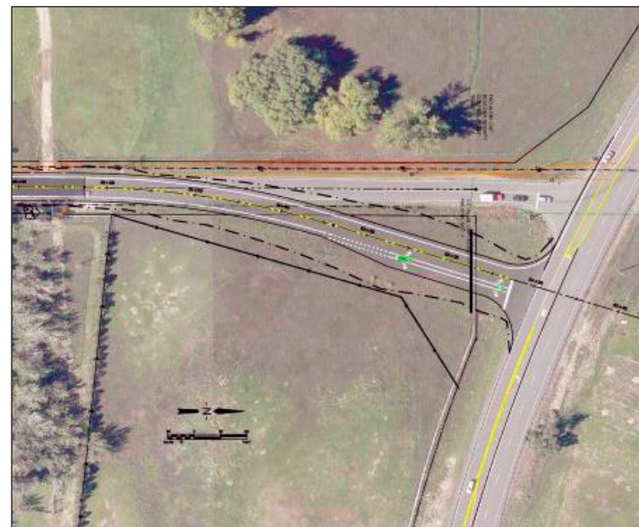
Phase 2 of the 71st Street project includes a wider road, with paved shoulders and a redesigned access to Highway 52. Phase 2 will begin sometime after Phase 1 has been completed.
